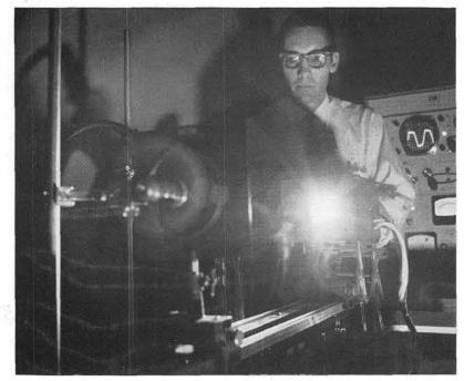
LAB-BUILT LASER (light amplification by stimulated emission of radiation) produces a thin, pure, hot, beam of coherent light. Charles E. Bates used the laser to check a theory about infrared transmission.
